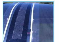
ITO film for EMI Shielding
